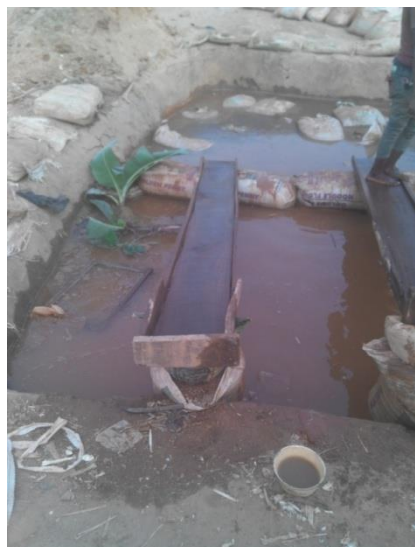
Fig. 7: Sluicing process at the Manyara river
