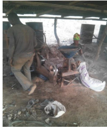
Fig. 4: Gold sample been ground using grinding machine at the processing site (Nassarawa Village)
